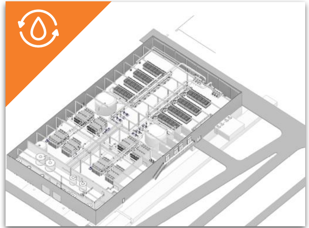
Layout plant - (capacity 2000-4000 m 3 /h, footprint 1 ha)
